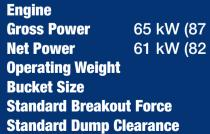
Yunnei YN38GBZ1 65 kW (87 hp / 88 ps) @ 2,400 rpm 61 kW (82 hp / 83 ps) @ 2,400 rpm 4,987 kg 1.0 m<sup>3</sup> Force 51.5 kN earance 2,567 mm
