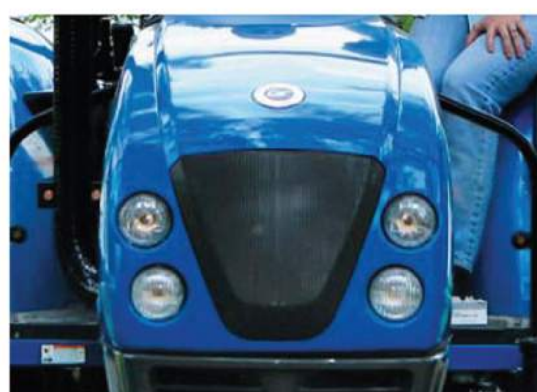
For improving the visibility working at day or night, TWO front work-lamps and TWO rear lamps are installed.
