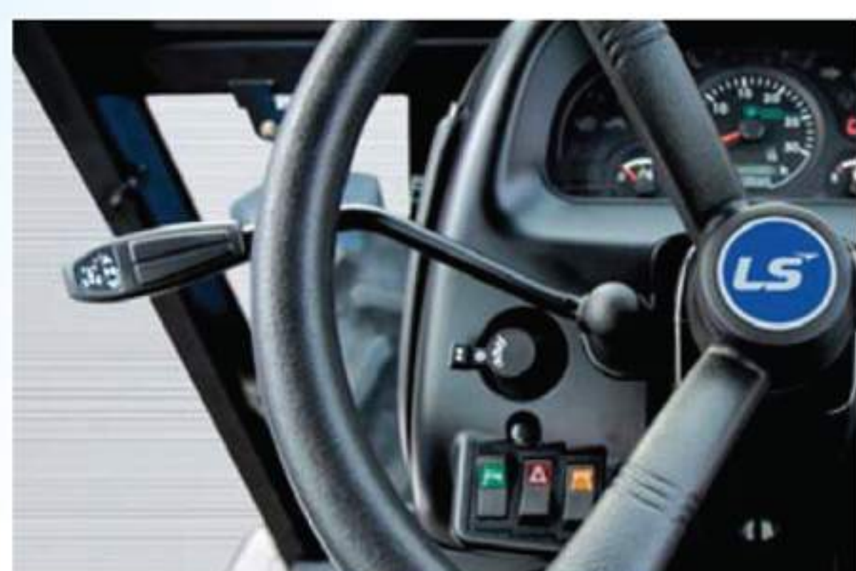
The superior finger-trip control type Shuttle Lever for forward/reverse shifting.
