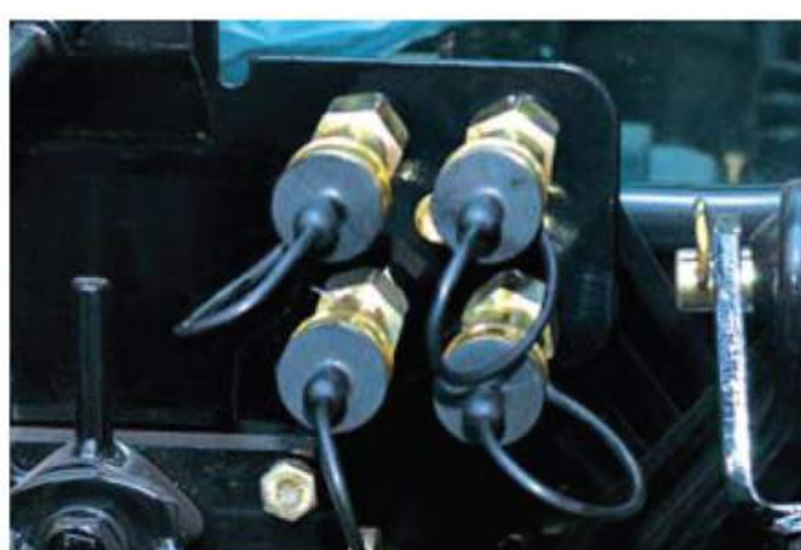
Open center system with 1 or 2 remote control valve to suit customer's needs at any time. Monoblock design valve.
