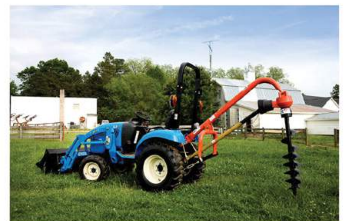
Can be equipped with various of attachments e.g. front end loaders, posthole digger and other implements to do many kinds of jobs.
