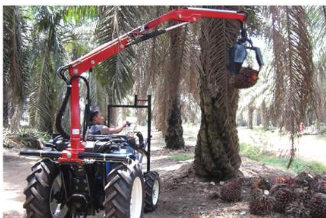
Suitable for mini crane grabber for infield / roadside collection in palm plantation
